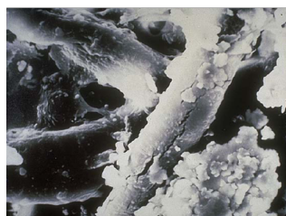
Degraded paper insulation
